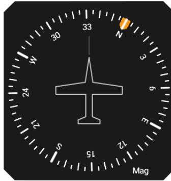
Figure 2.28: Illustration of the direction indicator.
