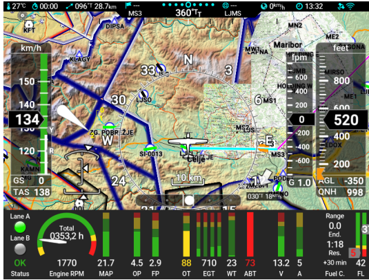
Figure 2.17: A moving map variant of modern screen.
