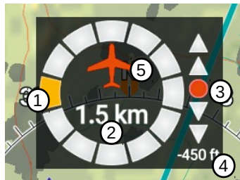
Figure 2.45: Threat classified as warning comes from left, distance is 1.5 km, about at the same visual level, 450 feet below.
