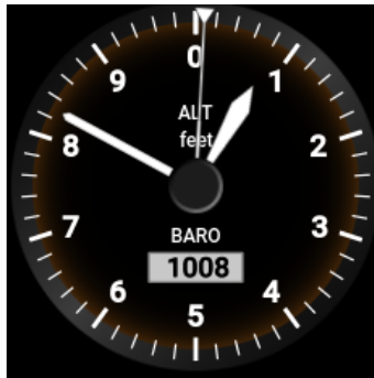
Figure 2.20: The altitude indicator with the scale given in feet. Three needles are shown in this case.
